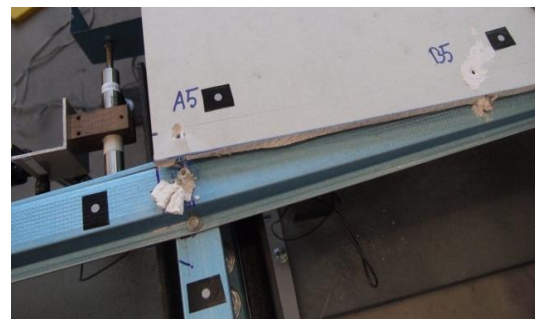
Figure 6: Tear-out of plasterboard at the screw connections located at the corners of the diaphragm
